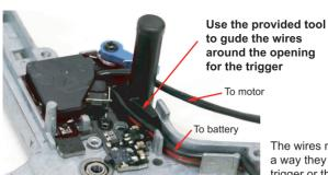
The wires must sit as low as possible in a way they do not stay on the way of the trigger or tha safety lever
