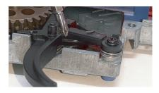
**8.** Check the clearence of the inner safety lever it has to moove freely. If needed change with the provided with the kit safety lever as it provides more clearence.
