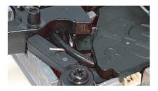
7. Install the trigger and check the wire clearence under the trigger. If needed push the wires down with a dull tool. The trigger has to move without rubbing into the wire.
