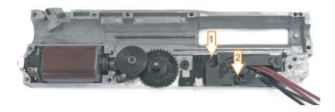
**5.** Install back the sector gear. When installing it make sure to position it in a way that the cam under it faces up (12 o'clock) as shown on the picture.
