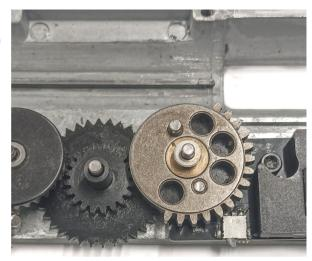
**6.** Make sure that the sector gear is shimmed in a way that dos not touch the ASCU board, and there is a proper engagement of the cut-off switch.
